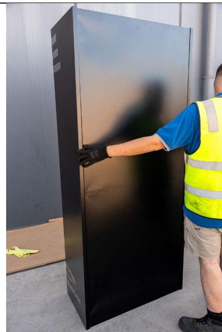
Fig. 19. Back panel slotted into the side panels.
