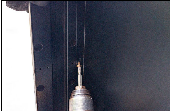
Fig. 32. Use a Phillips-head screwdriver to fasten the screw on the bottom panel (mid-section).
