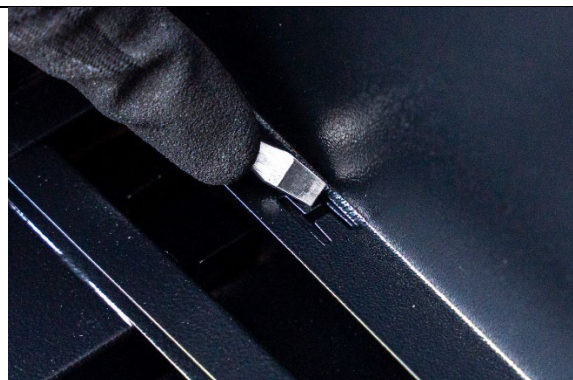
Fig. 28. Use a flat-head screwdriver to bend the H flaps into the frame.
