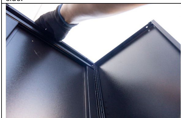
Fig. 12. Top view of side panel slotting into the door panel.
