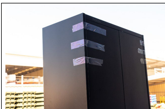
Fig. 14. Using heavy-duty tape can help in holding the side and front panel together.
